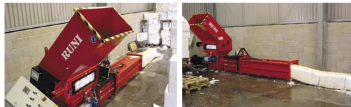
Details of some machines suitable for cold compaction or thermal densification
